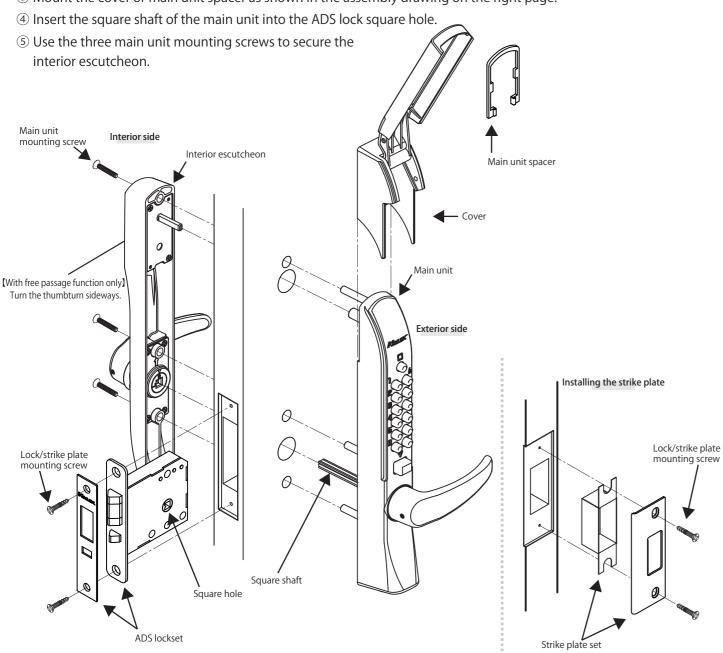
Drill holes for installing the KEYLEX main unit. (See the template of the KEYLEX main unit on the attached sheet.)
