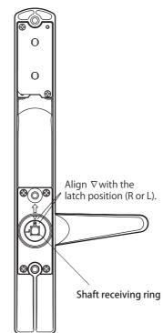
Mount the parts based on the door latch position. Check the latch position by viewing from the exterior side. Preparation for installation: Mount the parts based on the door later position. Check the lock functions properly. (Use a wedge or similar object to keep the door open.)
