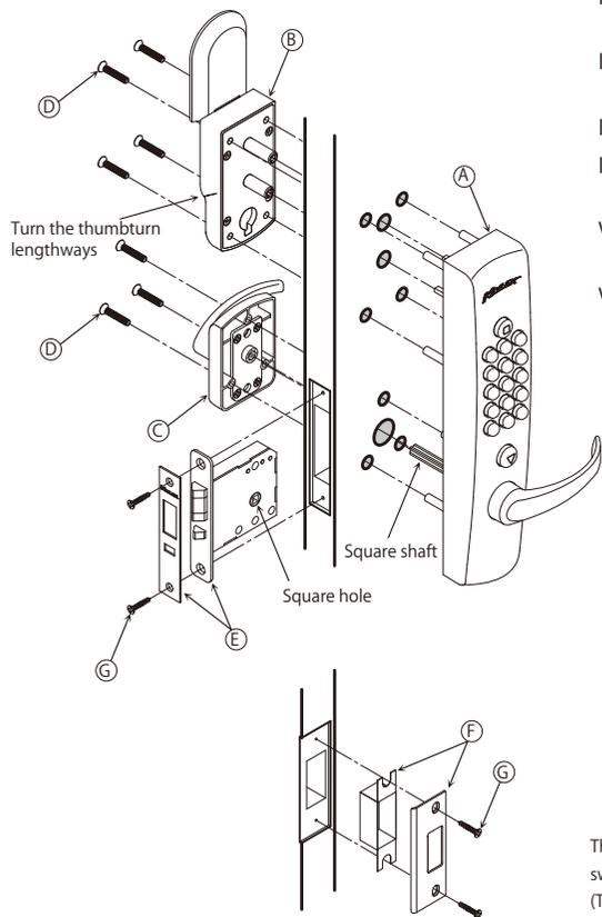
\* For the type with key, remove the key before installation.
