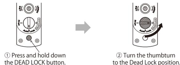
To switch from Dead Lock to Auto Lock, turn the thumbturn to the Auto Lock position. (Do not press the DEAD LOCK button.)
