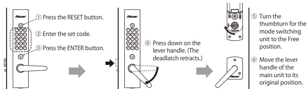
To switch from Free to Auto Lock, turn the thumbturn for the mode switching unit to the Auto Lock position while holding down the lever.
