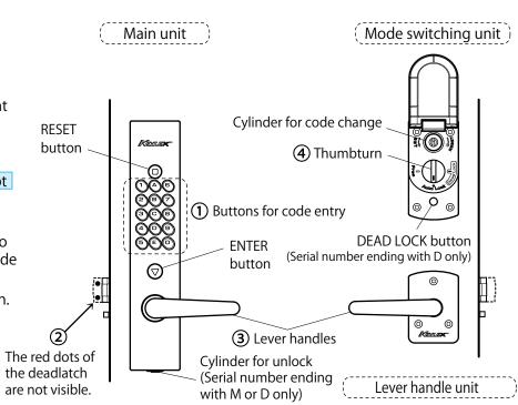
4 How the door is locked/unlocked from the exterior side depends on the position of the thumbturn. From the interior side, move the lever handle to unlock the door regardless of thumbturn position.
