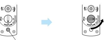
To switch from Dead Lock to Auto Lock, turn the thumbturn to the Auto Lock position. (Do not press the DEAD LOCK button.)
